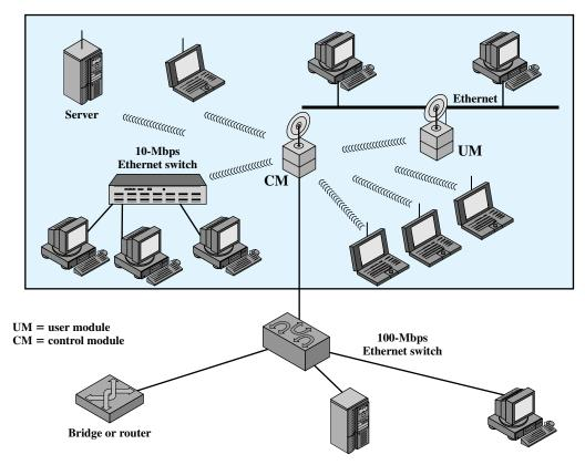
Figure 17.1 Example Single-Cell Wireless LAN Configuration
