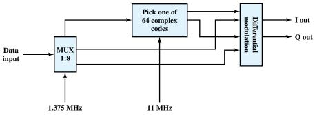
Figure 17.10 11-Mbps CCK Modulation Scheme
