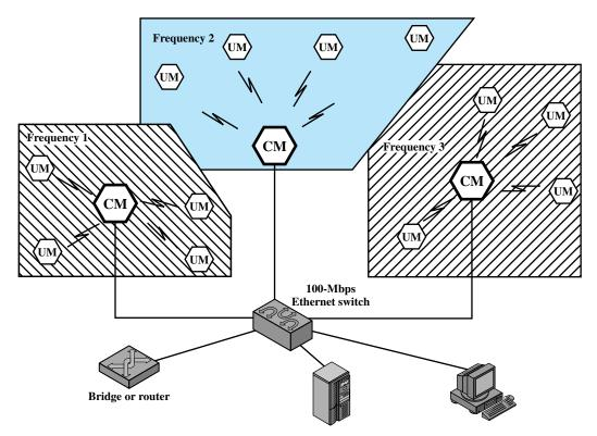
Figure 17.2 Example Multiple-Cell Wireless LAN Configuration
