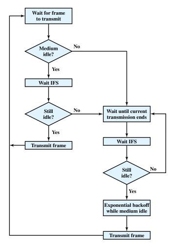
Figure 17.6 IEEE 802.11 Medium Access Control Logic
